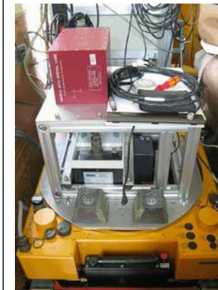
CASI and IR-Camera on stabilized platform
