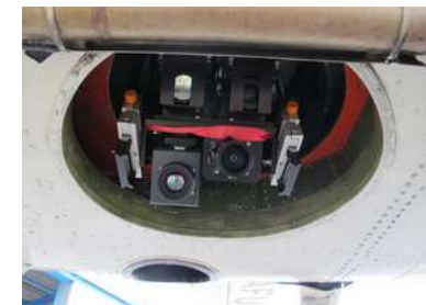
HySpex (GFZ Potsdam), IR- Camera (IGB/FUB), RGB- Camera (DLR)
