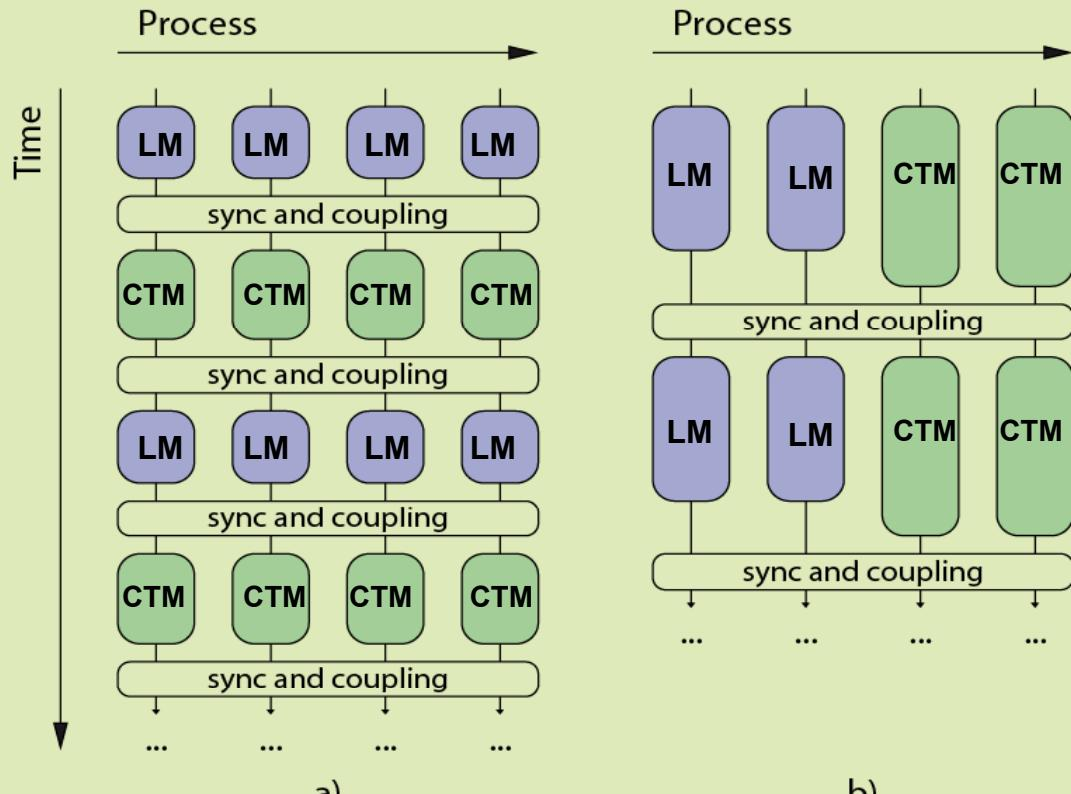
Coupling scheme for model systems: a) sequential, b) concurrent.
