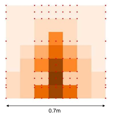
Concentration in the cross-section of the wind tunnel (dots are measuring points)
