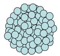
Clay particles form an aggregate of a coarser fraction
