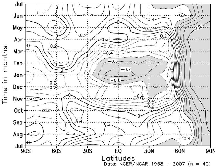
Fig. 11. Teleconnections (i.e., correlations) between the 100-hPa temperature at the North Pole and the zonal mean 70-hPa temperature ( $90^{\circ}\text{N}$ – $90^{\circ}\text{S}$ ) throughout the year. Shaded are correlations of more/less than  $+0.5/-0.5$  (NCEP/NCAR re-analyses, period 1968–2007).
