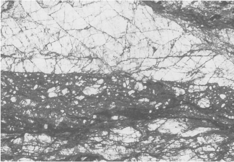
**Fig. 8.** Cataclastic microstructure of a type 2 shear zone. Note the angular, fractured clasts of partly serpentinized olivine (large clast at top, small clasts in matrix) and a nearly opaque matrix comprising mainly ultrafine grained serpentine and chlorite. View in the XZ fabric plane. Length of micrograph is 3.4 mm.
