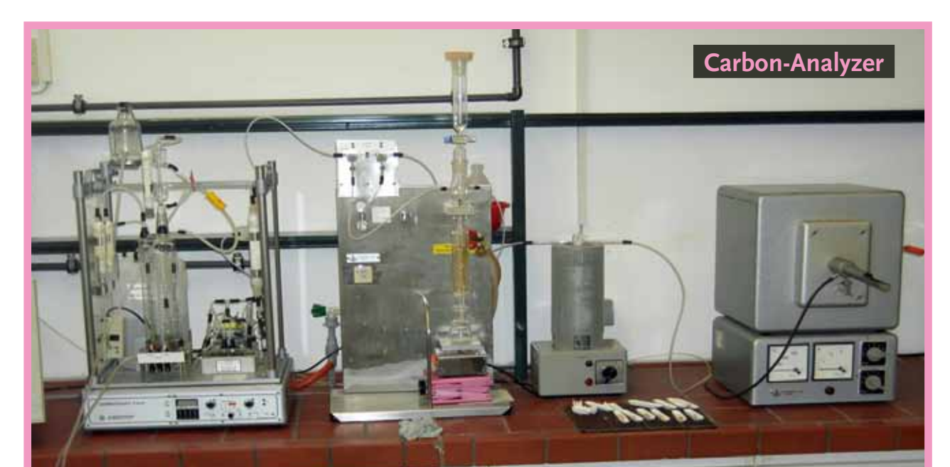
Fig. 7: The Carbon Analyzer used in the determination of organic and inorganic carbon contents
