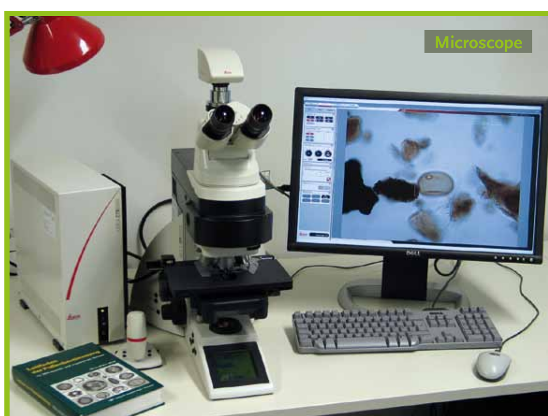
Fig. 1: After preparation the samples are analyzed at 500 – 1000 x Magnification. This may take ca. 1-4 d/sample
