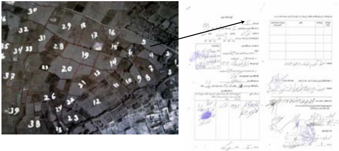
Figure 4: The village-based parcel register for private land as managed in the GIS: each individual parcel is digitized and linked with its parcel form signed by owners and witnesses
