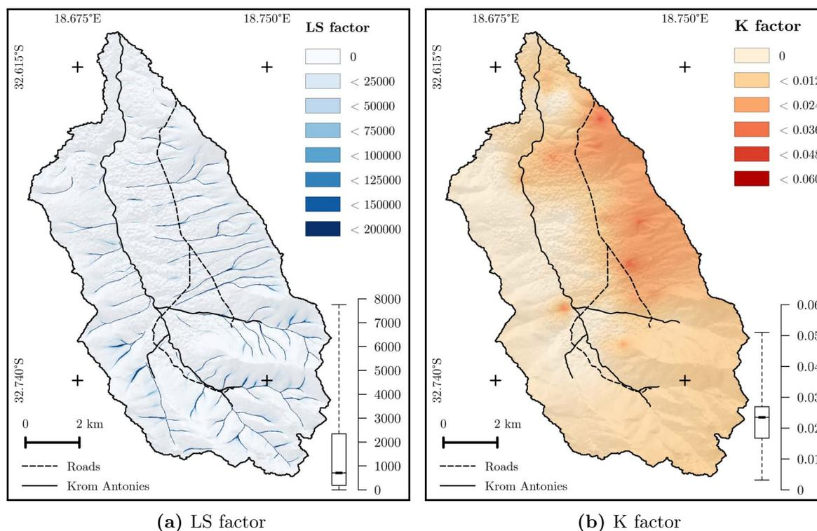
**Figure 5.6:** The resulting slope length and slope steepness (LS factor) with  $m = 1.6$  and the soil erodibility (K factor).
