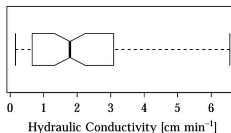
**Figure 5.9:** Boxplot of the hydraulic conductivity. Four outlying values are not covered by this plot.
