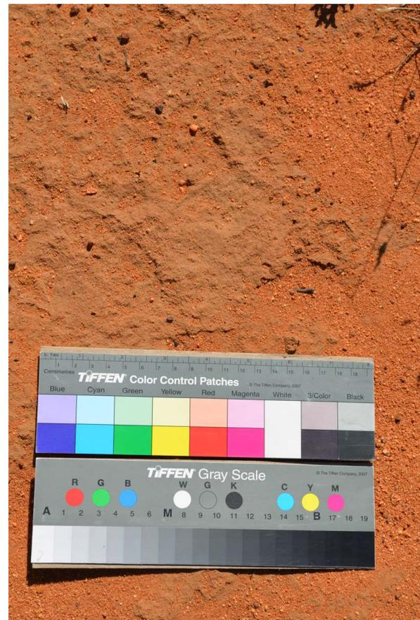
**Figure 4.2:** Example of a top soil picture and the corresponding color separation chart.
