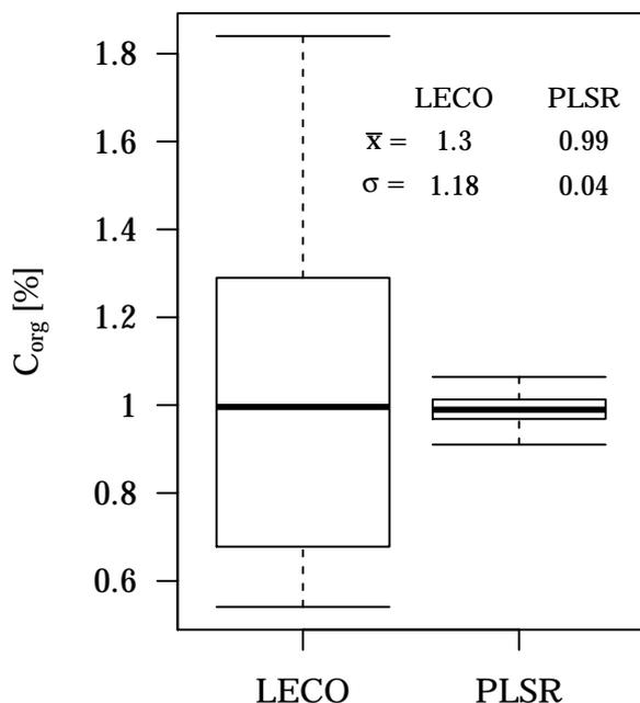
**Figure 5.10:** Comparison of the organic carbon estimated in laboratory via TruSpec CHN-S-Analyzer (LECO) and estimated using a regression model (PLSR).
