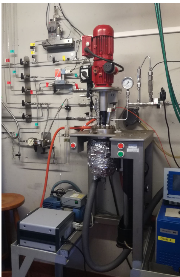
Fig. 5 High-pressure reactor system at the JKU Linz (Credits: Patricia Pappenreiter, JKU Linz)
