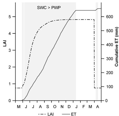
**Figure 3.** Modified forest growth allows for soil water limited evapotranspiration (ET): total (green and brown) leaf area index (LAI), cumulative evapotranspiration (ET), and periods (gray shaded) when soil water content (SWC) is above permanent wilting point (PWP) of an exemplary forest HRU from May 2001 to April 2002.
