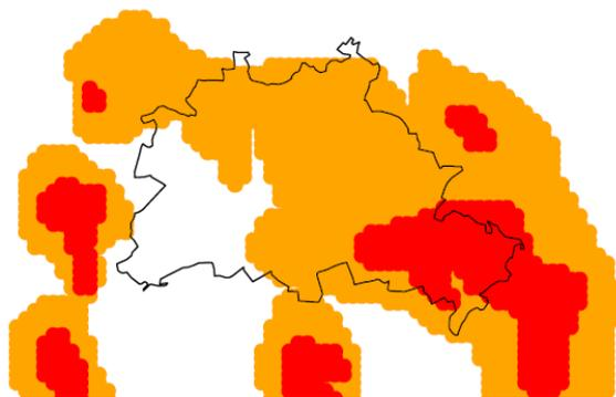
Fig. 2. Derived "footprint" for the 6<sup>th</sup> of June 2011 comprising the local hazard strength on a regular 1x1km grid.
