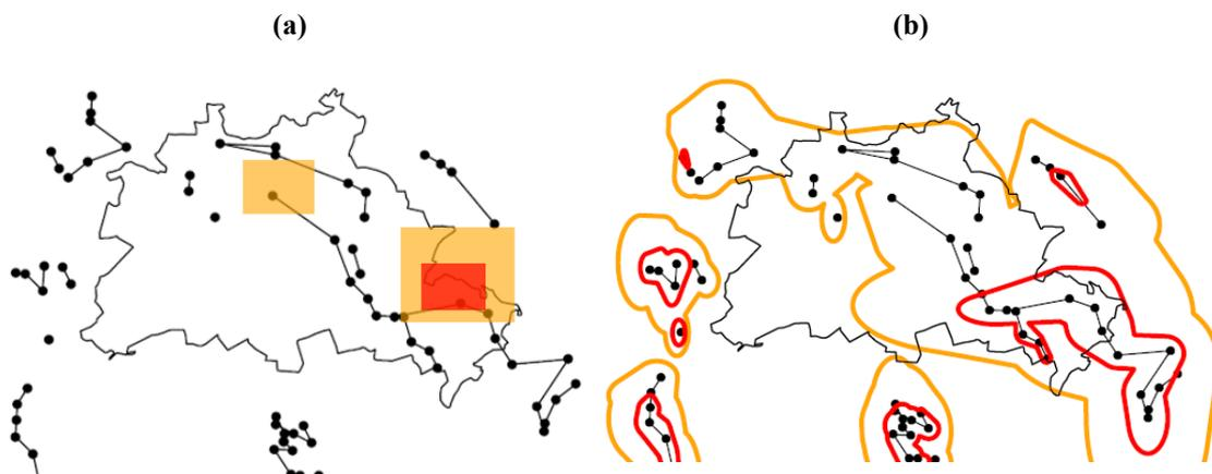
**Fig. 1.** Derivation of information on the local strength of the meteorological hazard for an example situation, the 6<sup>th</sup> of June 2011. (a) Original data from KONRAD analyses. Cell locations are shown as black dots. Information about the extent of areas with radar reflectivity >46dBZ (yellow) and >55dBZ (red) are shown exemplarily for 2 cells. (b) Derived polygons representing the envelope of the areas affected by >46dBZ (yellow) and >55dBZ (red).
