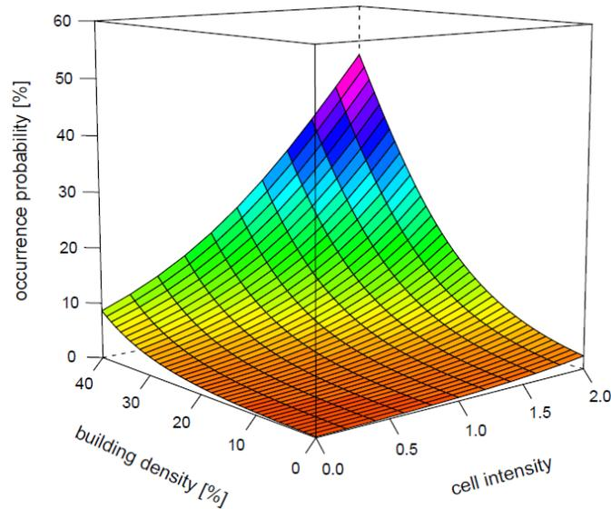
**Fig. 5.** Results of logistic regression model for the occurrence probability for water-related operations within a grid cell. Cell intensity of 0 corresponds to a radar reflectivity below 46dBZ, cell intensity of 1 corresponds to an exceedance of 46dBZ and cell intensity of 2 corresponds to an exceedance of 55dBZ.
