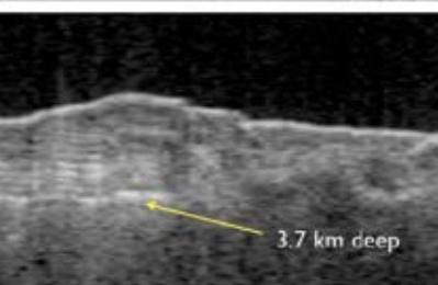
Looking through the ice deposits at the south pole with MARSIS. The corresponding ground track is shown above. (ESA/NASA/ASI/JPL Caltech/Univ. Rome)
