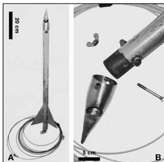
**Fig. 2:** Rocket-like bore probe for efficient collecting of benthos samples. **A:** General view. **B:** Detail of the removable head.
