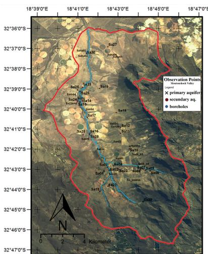
Figure 1: Selection of the Observation points in the study area. The black crosses are showing the position of shallow boreholes which only reaches the first aquifer about up to 20 m depth as well as river- and dam samples. The red dots are the positions of the boreholes deeper than about 20 m which reaches below the clay layer into the second aquifer. The map is based on LANDSAT images, edited with ArcGIS and image editing software.
